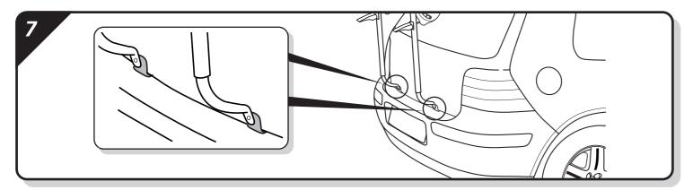
Hook the feet under the bottom of your tailgate. In some cases it may be necessary to slightly open the tailgate to enable the feet to
